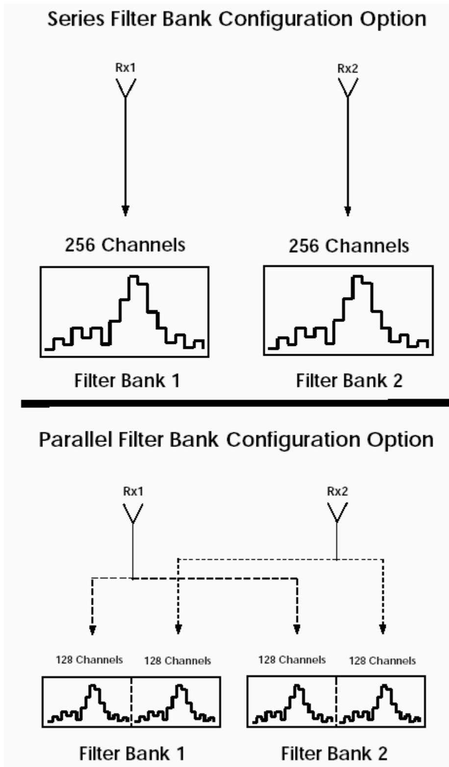
**Figure 5.1:** The filter bank parallel and series configurations.
